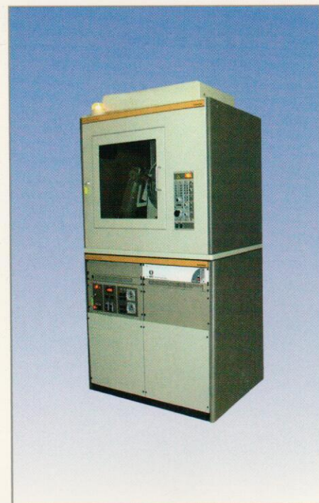
122D Upgrade fitted to Siemens D500 Diffractometer
