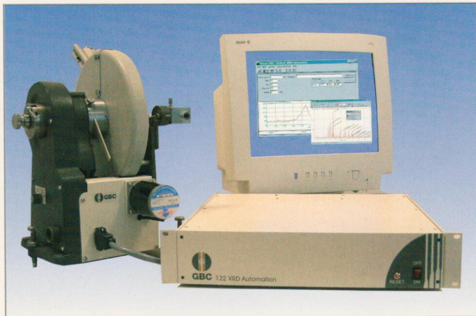
122D Upgrade added to Philips PW 1050 goniometer
